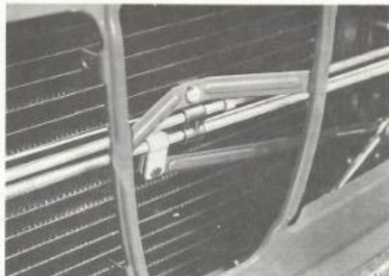
CENTRAL BUSHING FIXED WITH TENSION PIN, MODEL 1973
