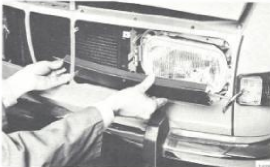
REMOVING THE PROTECTIVE PLATE, AS FROM MODEL 1974
